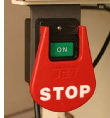
The large paddle-style OFF switch makes it easy to shut the ProShop saw off by hand or with a bump of your leg.
